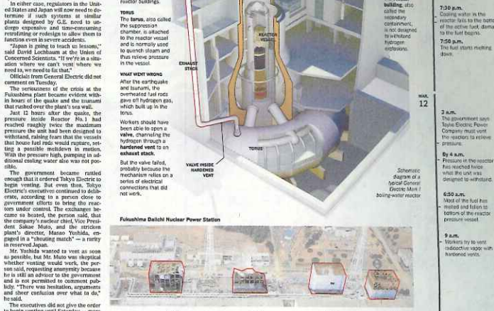
Source: Tokyo Electric Power Co., Fukushima Daiichi Nuclear Power Station. Diagram of a typical General Electric Mark I boiling-water reactor.
