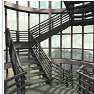
In 1989, the "Stair Tower, Rhodes Hall, Cornell University," by Keith Howie and Ben Trumbore, was rendered using distributed ray-tracing to create soft shadows. It took one hour to compute on eight HP835 workstations.
