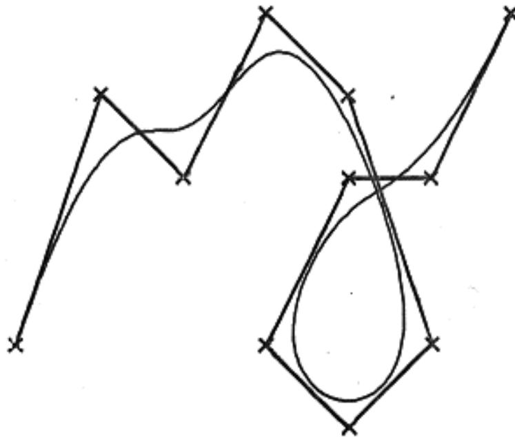
Figure 17 – Open cubic ( $M = 4$ ) B-spline curve defined by the polygon from Figure 7.
