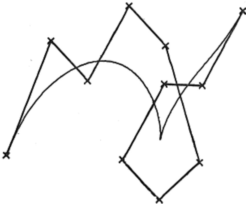
Figure 7 – Example of a Bézier curve for a 10-sided polygon.
