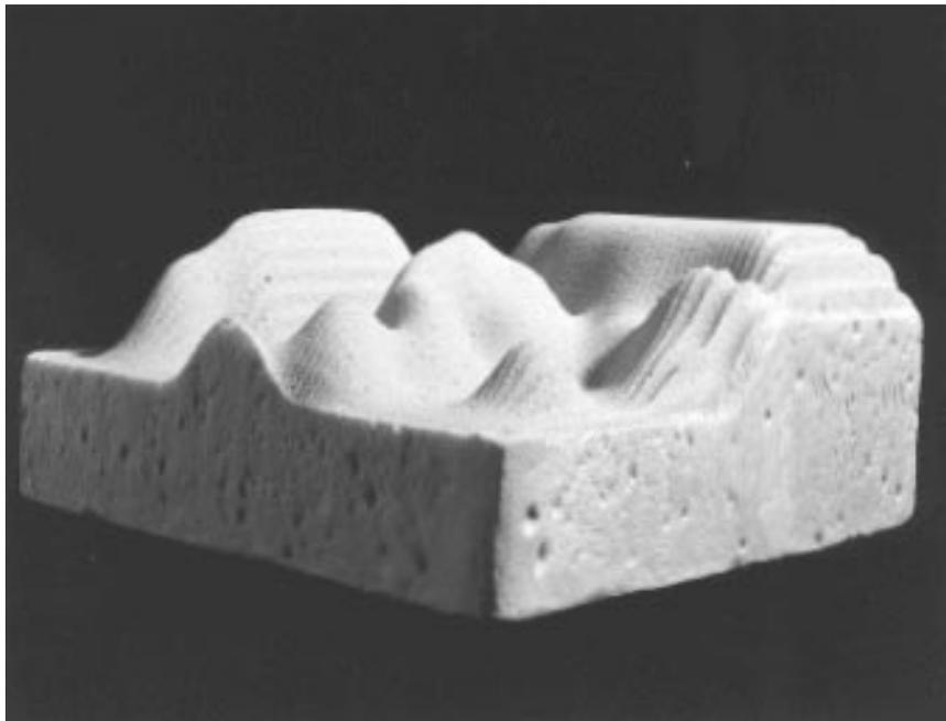
Figure 32 – Pictures of a complicated B-spline surface cut by a numerically controlled milling machine.
